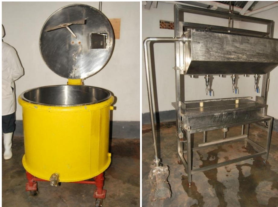
Figure 6. Boiler and fermentation tank (left); and filling and sealing machine (right)
